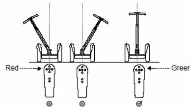
When the center Balance Indicator light is green, the Segway PT is ready for you to step onto the Mats.
